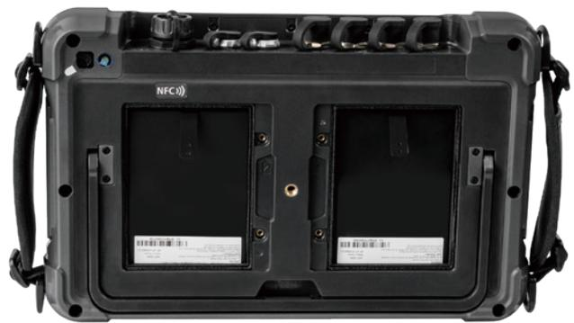
Dual batteries provide 8-10 hours continuous operation.
