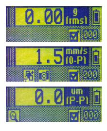
For those precision machines that have very low vibration levels, a precision reading is necessary. In addition to an extra quiet accelerometer that is supplied as a standard accessory, both vPod and vPod II incorporate a built-in gain circuit to amplify small vibration signals and show the reading in precision mode when you turn the gain mode on. This one button gain function allows the user to increase precision by one decimal place.
