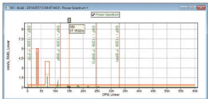
Show or hide alarm levels and fault frequencies on a spectral plot
